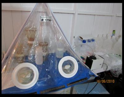
Samples filtered in field with 0.45 µm membranes (celulose acetate) – Dissolution of membranes for recovery of suspended matter (SM) – HNO<sub>3</sub>, H<sub>2</sub>O<sub>2</sub>, HF & HCl 6N
